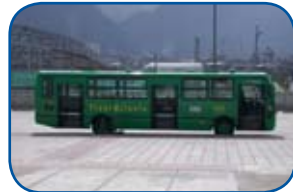
Additional doors on feeder line—Bogotá, Colombia
