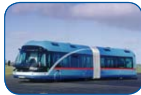
Specialized BRT Vehicle—Translohr
