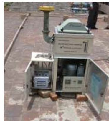
Figure 2: Conventional (offline) air monitoring equipment
