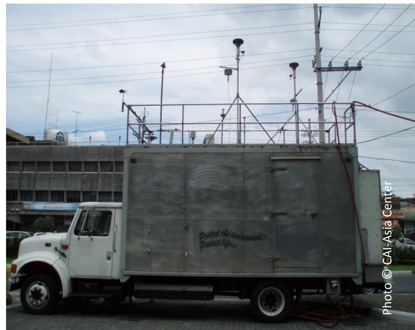
PHOTO LEFT Automatic air quality monitoring station in Cebu City. This is operated by EMB – Region 7.
