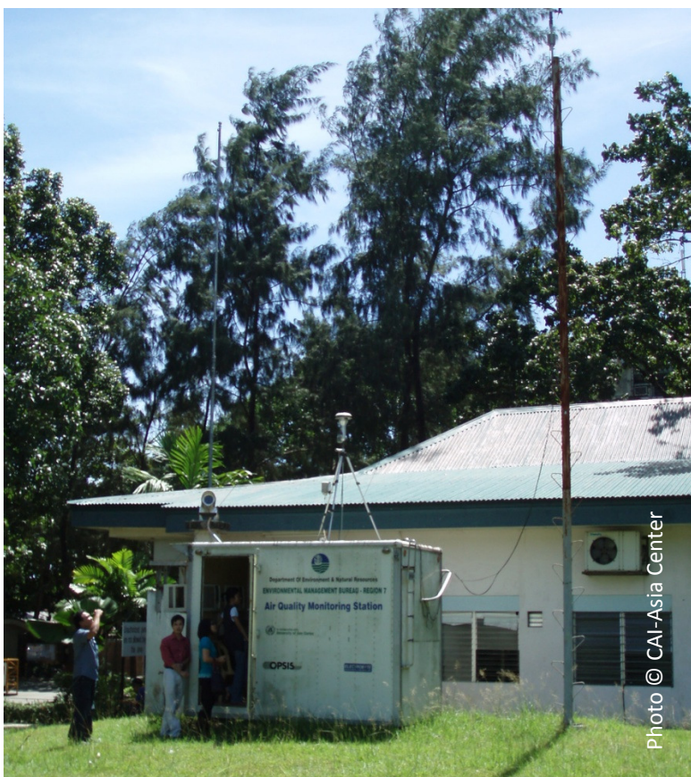
PHOTO BELOW Mobile air quality monitoring station in Metro Manila. This is operated by the Environmental Management Bureau – National Capital Region (EMB-NCR).
