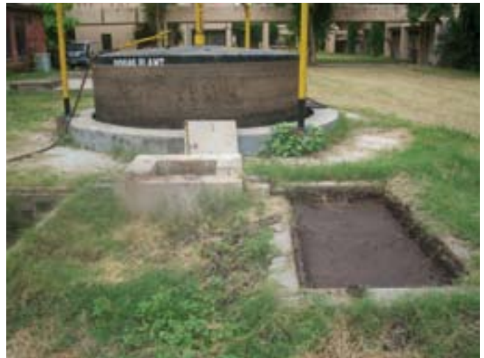
Figure 4b A pictorial view of same biogas plant after three day of feeding of de-oiled seed cake
