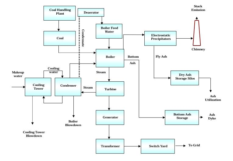
Figure : 2.3 Process Flow Diagram
