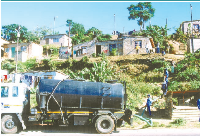
Figure 9: Problems of access by conventional desludging vehicles
