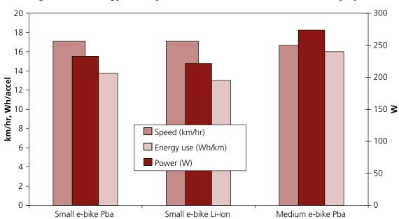
Figure 4.18: Energy Used by Small and Medium Electric Bikes in City Cycle
