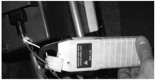
Figure 4.7: Current Measuring Device Clamped on the Battery's Hot Wire
