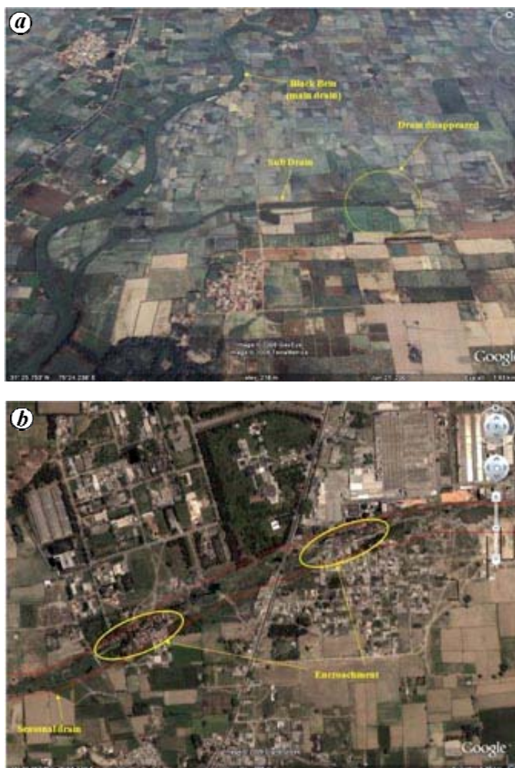
Figure 1. Google Earth images of encroached drains in (a) Kapurthala District and (b) Hoshiarpur city.
