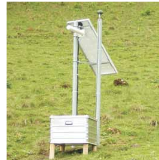
Figure 2b: GNSS SN (Novatel Smart Antenna, WLAN-Antenna, solar panel, alu-box with battery, charge controller and wireless device server).
