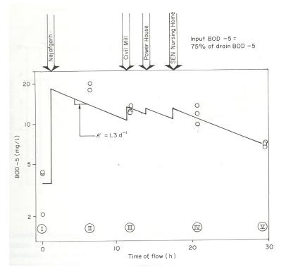
Fig: A 3.4 Observed (O) and calculated (-) BOD-5 profile at five sampling stations between Wazirabad and Okhla
