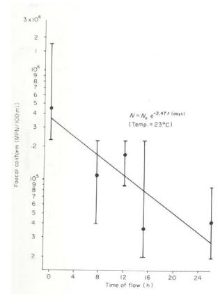
Fig. A 3.1 & A 3.2 : Disappearance of fecal coliforms in the Gurgaon
