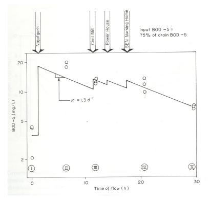
Fig. A 3.3 Observed (O) and calculated (-) BOD-5 profile at five sampling stations between Wazirabad and Okhla
