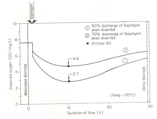
Fig. A 3.5: Predicted DO profiles for reduced BOD loads at 30 °C
