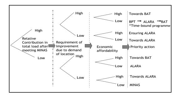
Figure 6.1: Guiding tool to decide level of Control Technology
