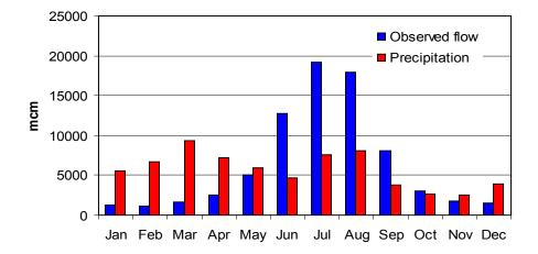
Figure 3. Mean monthly precipitation (modified) and observed flow in the Tarbela catchment (Upper Indus Basin).
