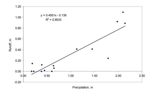
Figure 21. Annual average runoff/area as a function of annual average precipitation (or modified precipitation). See Section 3d and Table 2 for catchments of the Indus Basin.
