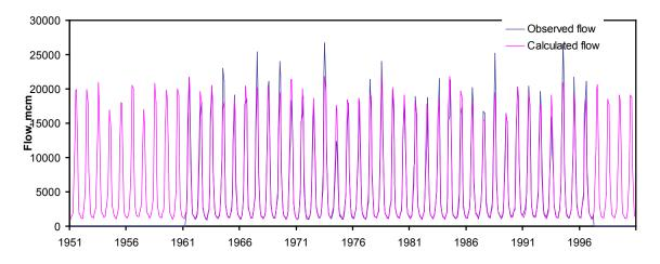
Figure 5. Observed and modelled flow at Tarbela.
