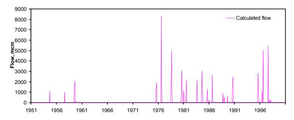
Figure 13. Modelled flow from the Ravi catchment.
