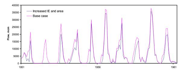
Figure 21. Impact of increasing irrigation efficiency from 0.4 to 0.6 and increased irrigation area by 10% on flows at in the Indus River at Kotri.
