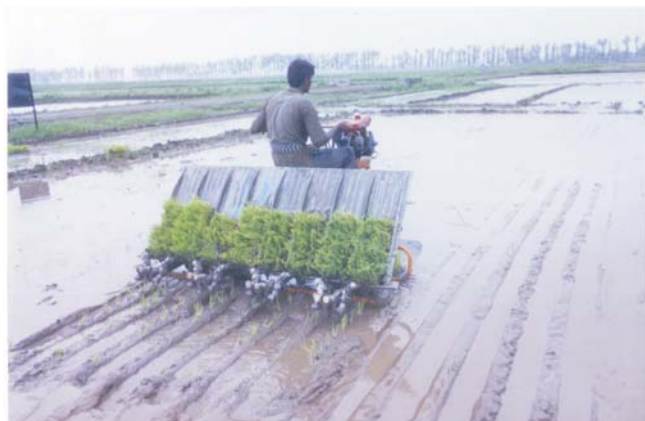
Figure 1. A mat-type rice transplanter in operation.
