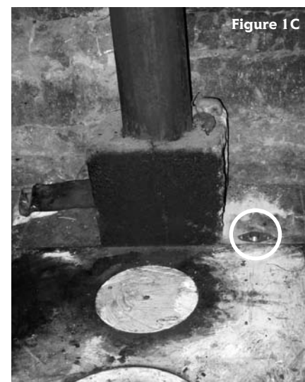
Figure 1. The temperature logger used as SUMs in this study (A), downloading SUMs data after deployment with a PDA and field readout interface (B), SUMs placed in the back of the Plancha stove surface (C) (Photos: I. Ruiz-Mercado)
