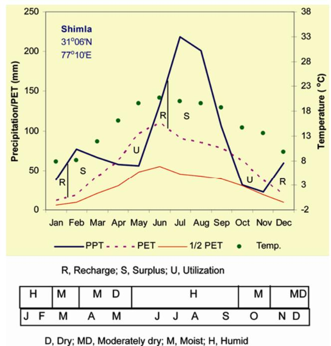
**Figure 2.** Water balance diagram.
