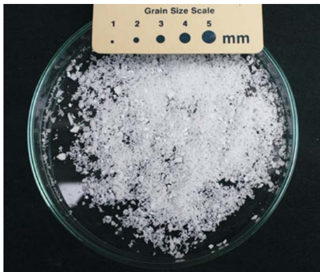
Figure 3. Epsom crystals developed from FCT.
