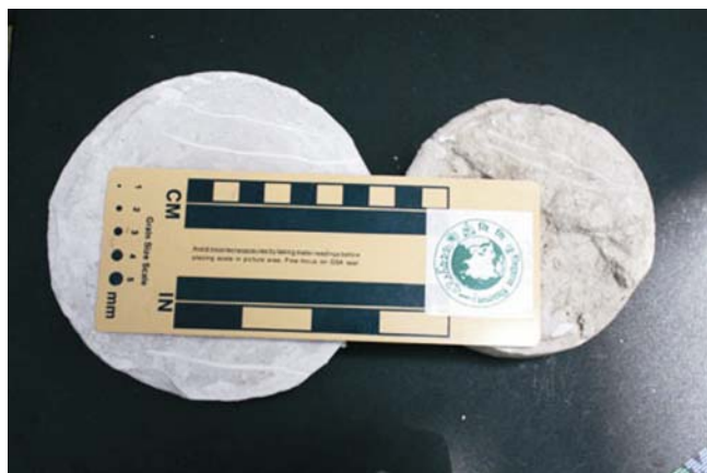
Figure 4. Cakes of fine grained gypsum dried in solar dryers.
