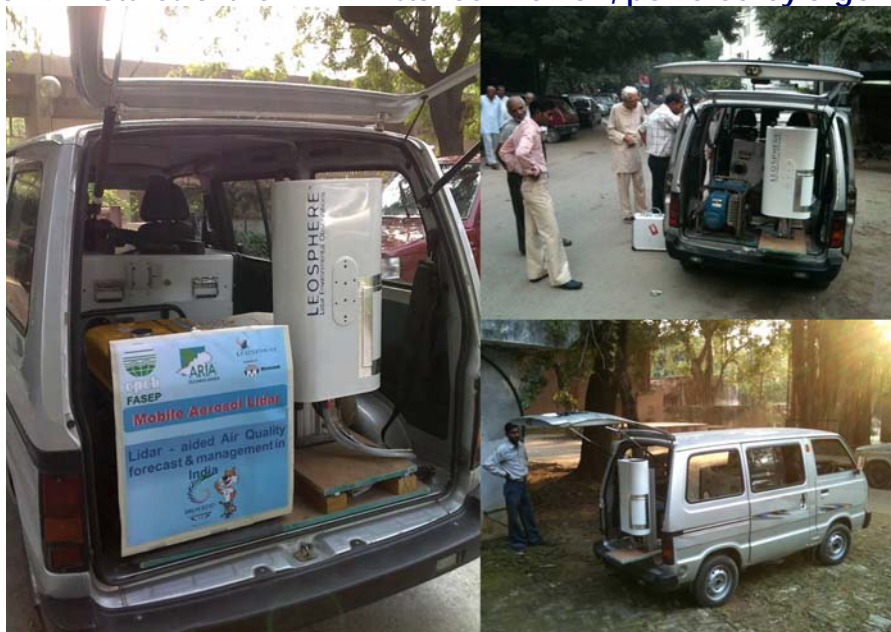
Figure 19: Pictures of the LIDAR installed in a van, powered by a generator
