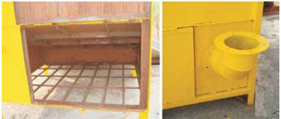
**Figure 2** Photographs of a fireplace with chimney outlet on side
