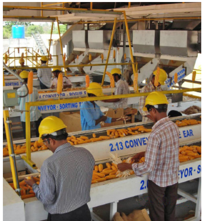
Picture 9. Monsanto's corn processing facility- sorting of wet ears, Shameerpet, Andhra Pradesh
