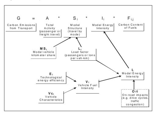
Figure 3: ASIF Equation in Two Dimensions for Carbon Dioxide Emissions
