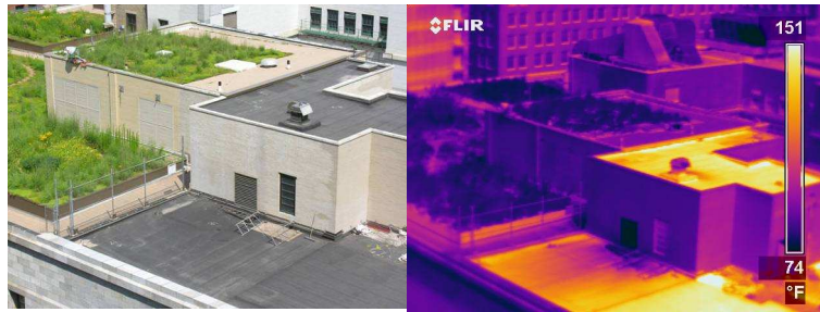
Heat sensing pictures illustrate the major temperature difference between green roofing on Chicago's City Hall (left) and traditional roofing (right)
