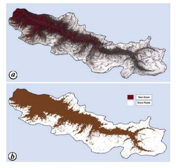
Figure 2. *a*, AWiFS sensor data for 14 May 2007. *b*, Snow pixels identified by NDSI method from AWiFS sensor data for 14 May 2007.
