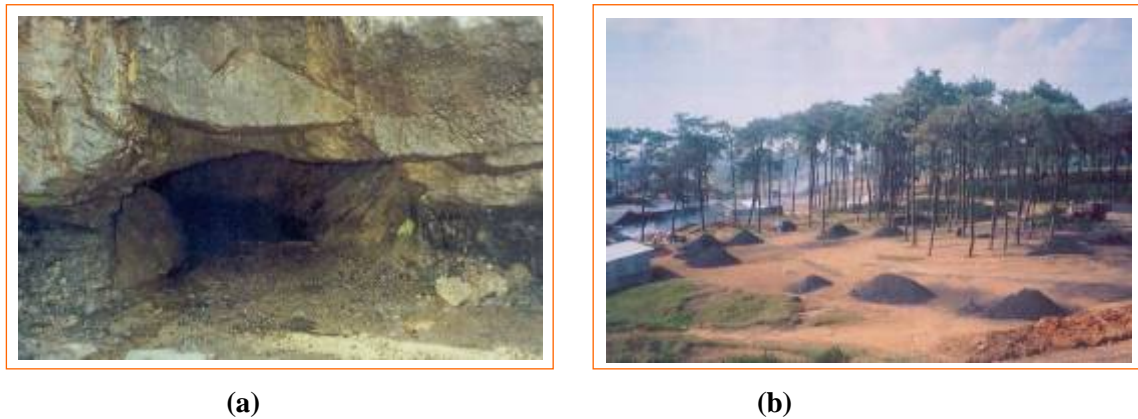
Figure 1.1: Rat-hole mining method - a crude mining technique is the sole method of coal extraction in the district (a). Damage to natural vegetation due to piling of coal (b).
