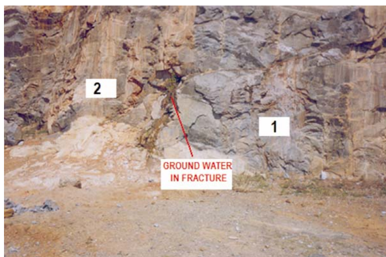
Figure 1. Occurrence of groundwater in deeper fracture in hard rock.
