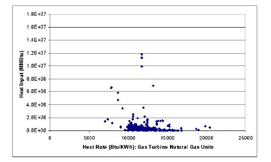
Figure 11. Natural Gas Turbine—Heat Input–Weighted Heat Rates
