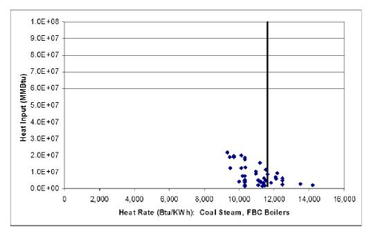
Figure 6. Coal Fluidized Bed—Heat Input–Weighted Heat Rates
