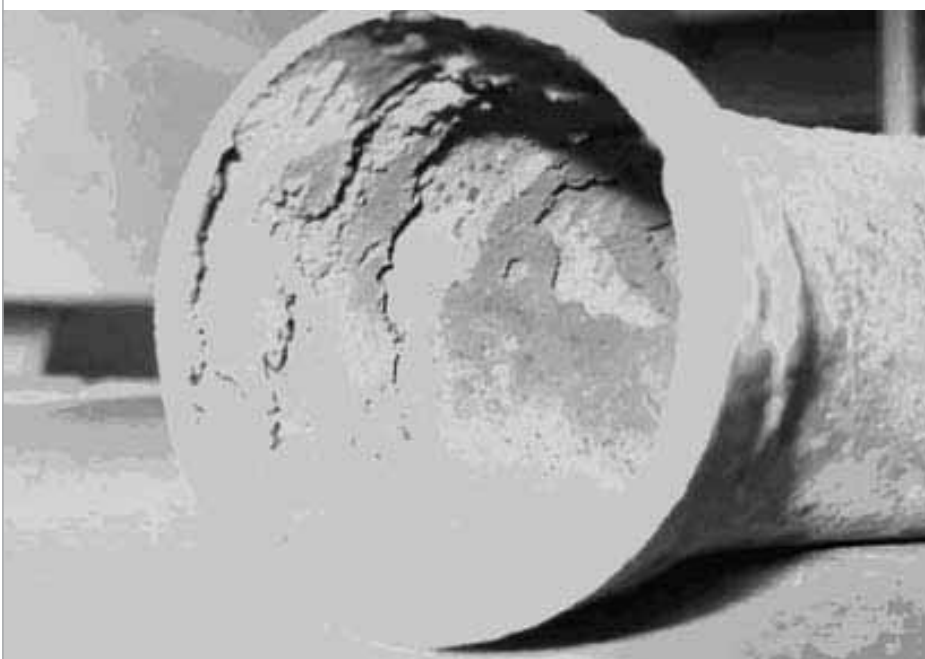
Figure 2: Pipe corrosion caused by carbonic acid
