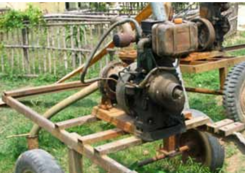
Figure 15: Pumping sets placed on a handcart
