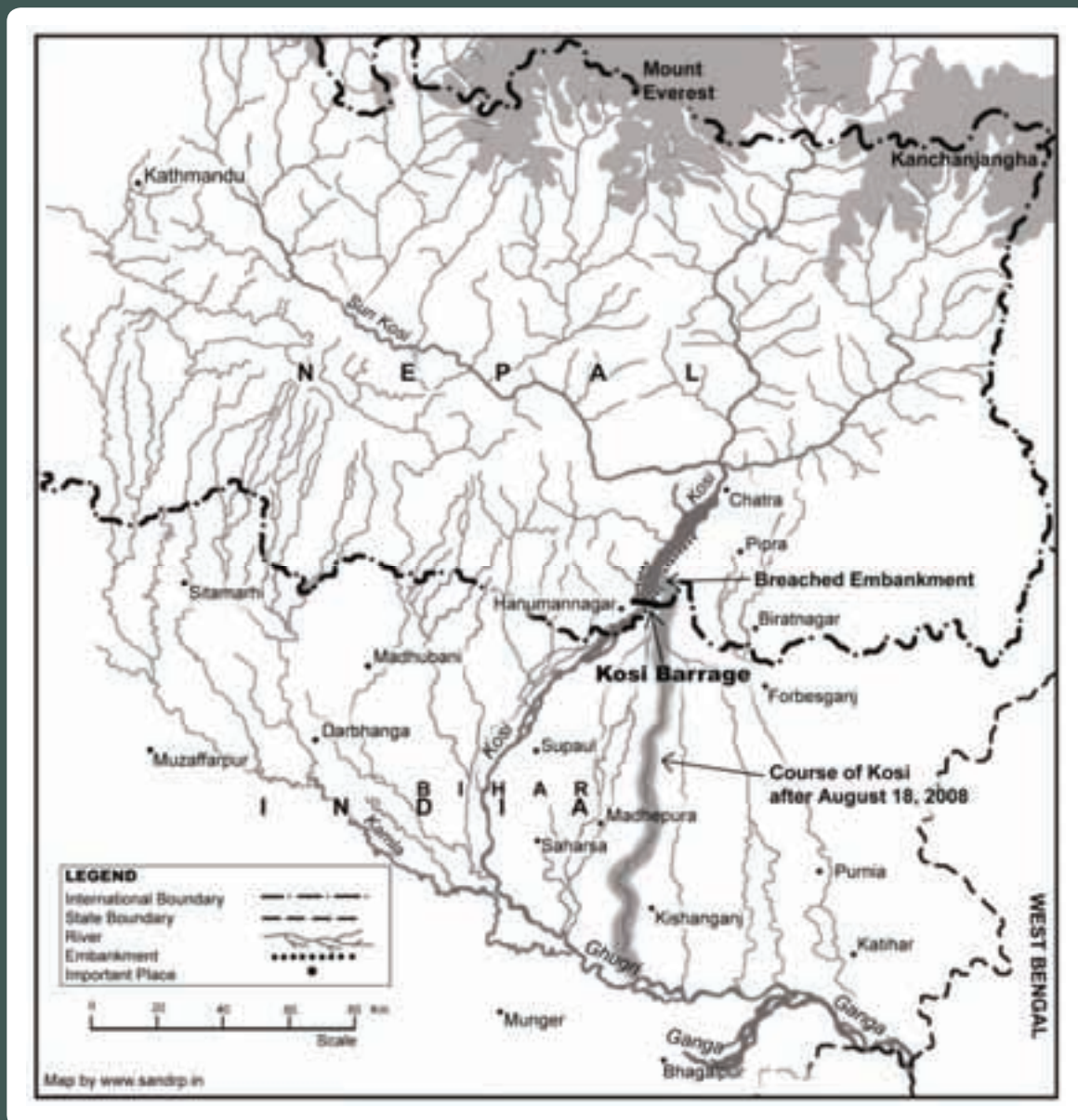
Figure 4: Present course of the Koshi after the 2008 embankment breach
