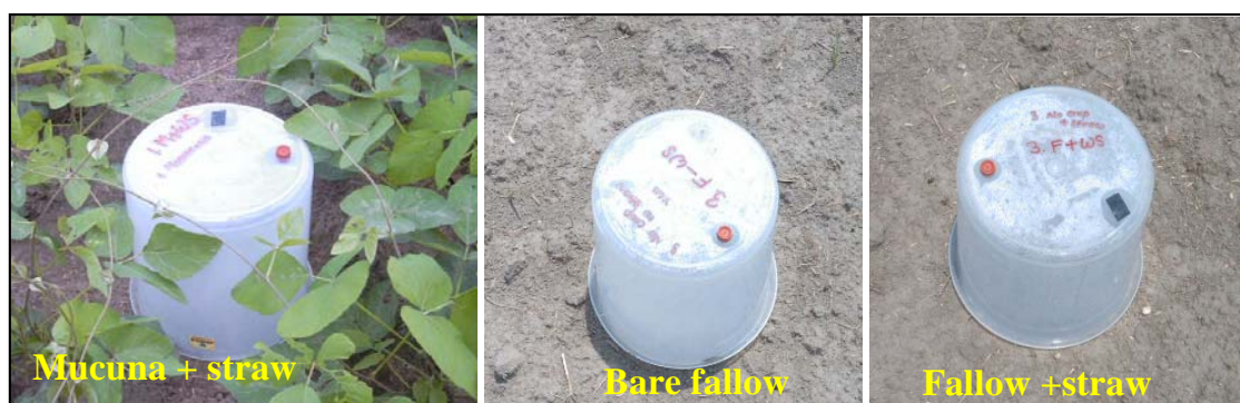
Plate 2. Installation of gas collection chambers in the field plots (on/station field experiments, Rampur, Chitwan province, Nepal, 2003).
