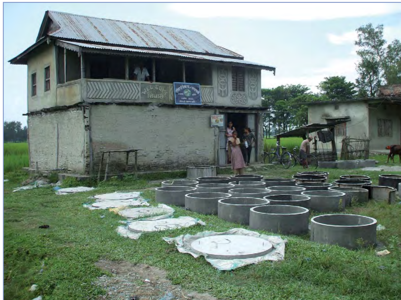
Photo 3: Darbesha WSUC office Concrete rings and slabs can be seen in the foreground
