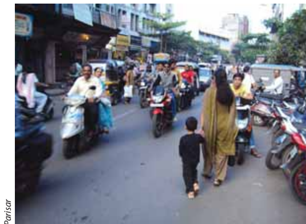
Fig. 9: High level of pedestrian-vehicular conflict due to missing or unusable footpaths
