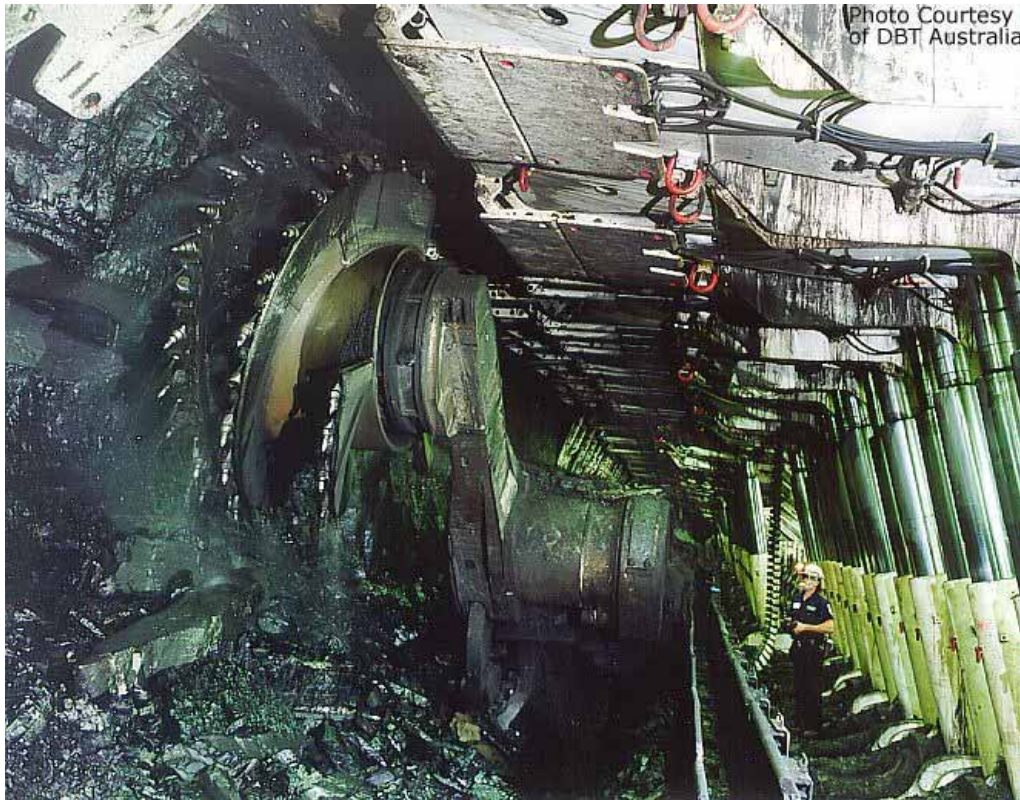
Figure 9: An Operating Longwall Face
