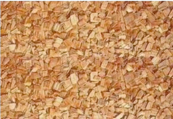
70 Figure A14: Wood chips. Enzymes can help softening the woodchips and save energy in the refining process.
