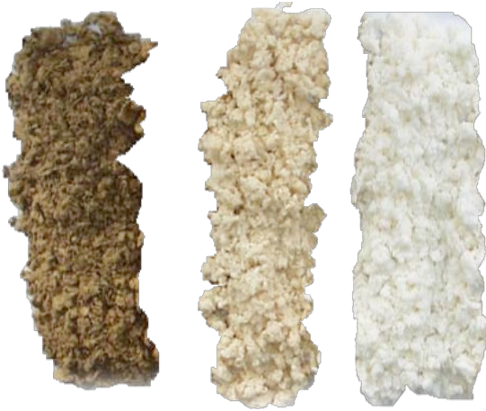
Figure A13: Non-bleached pulp (left), semi-bleached pulp (middle) and bleached pulp (right). Enzymes can boost the bleaching process and reduce chemical use and emission of greenhouse gasses.
